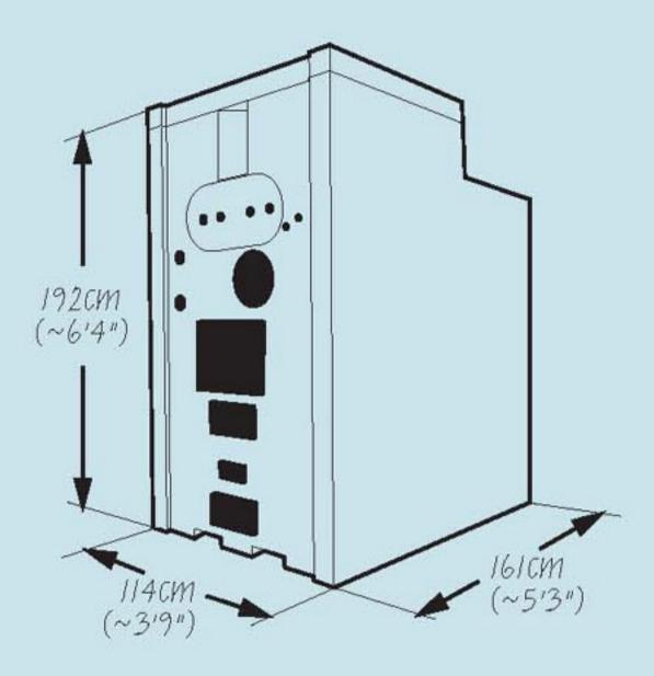
Flue gas exit diameter: 219 mm external, 206 mm internal. Recommended length of flue gas tube (chimney): 4 m.
